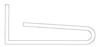
1mm thick aluminum - cold formed sheet strip
